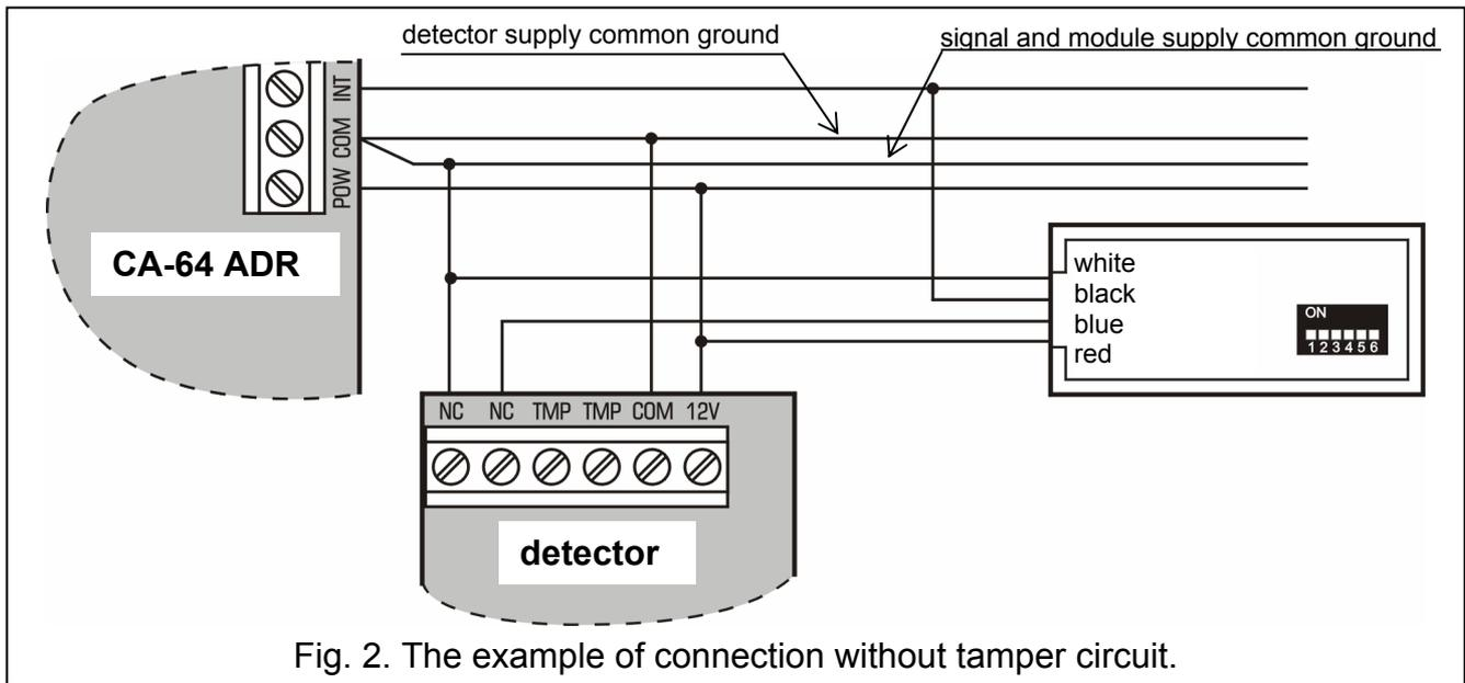
Fig. 2. The example of connection without tamper circuit.
