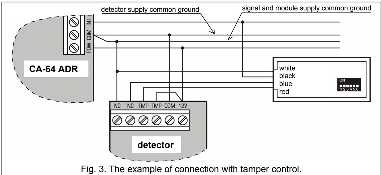
Fig. 3. The example of connection with tamper control.
